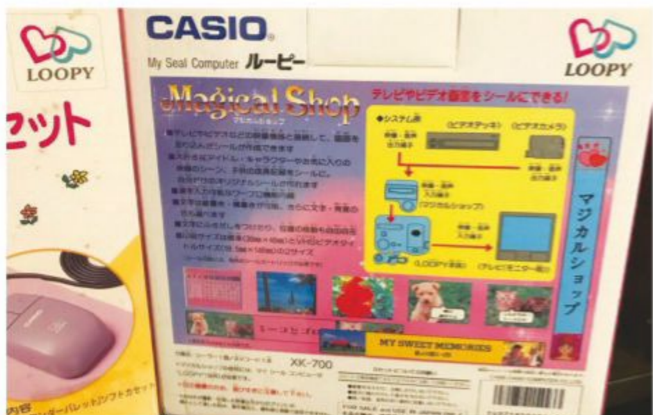
» The Magical Shop let you connect the Loopy console to a VCR or camcorder.
